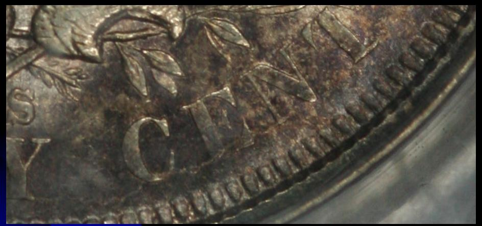
Die Crack Below C E N (Others report die cracks i) Through T in cents & ii) Above U N I T E D)
